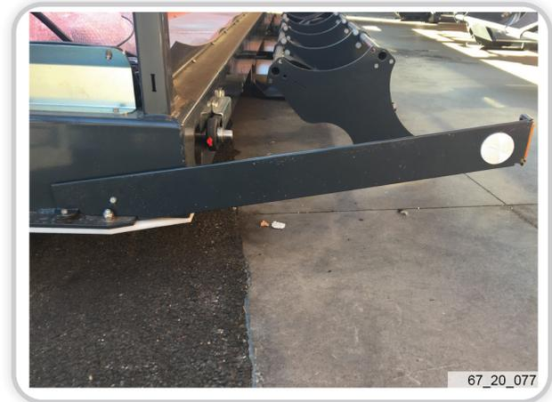
**► BLOCAGE DU TIMON AVEC UN AXE MECANIQUE**
