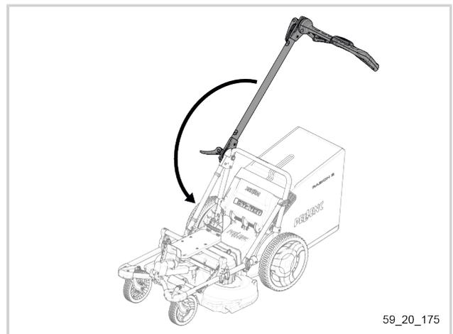
6. Lock the handlebar adjustment lever (5) by pulling it forwards.
