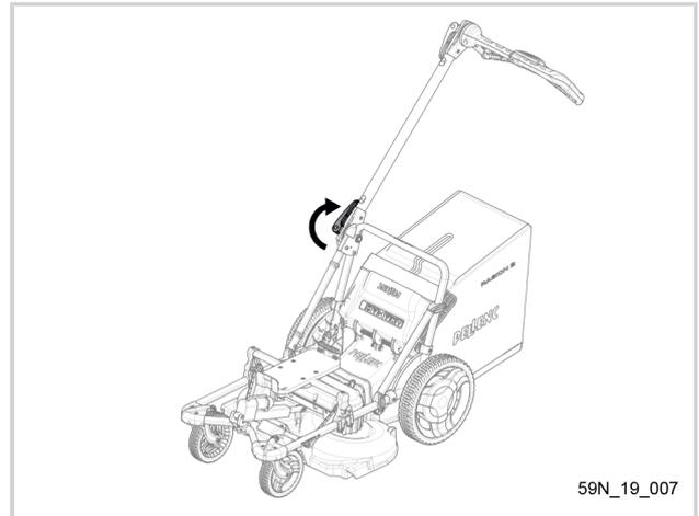
Unlock the handle adjustment lever (3).
