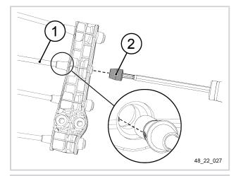
Using a torque screwdriver and a TORX 20 bit, tighten the new prong fastening screw.
