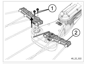
4. Using a TORX 20 screwdriver, remove the prong attachment screw.
