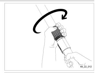
2. Adjust the length of the telescopic pole according to the working height.
