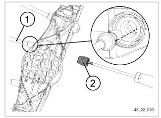
3. Using a torque screwdriver and a TORX 20 bit, tighten the new prong fastening screw.
