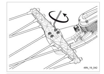
2. Using a TORX 20 screwdriver, remove the prong attachment screw.
