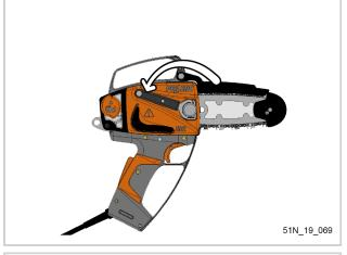
Checking the tension of the chain
