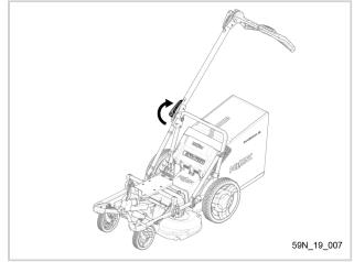
Unlock the handle adjustment lever (3).
