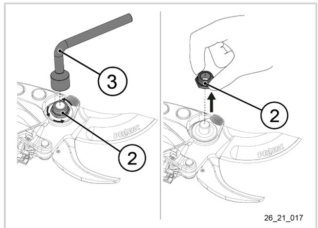
5. Unscrew the nut (2) with the supplied wrench (3) and remove the nut (2).
