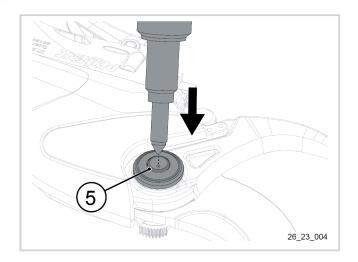
14. Grease the blade shaft (5). See Section 6.6, "Greasing the blade".
