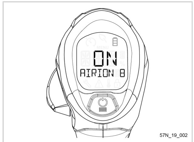
4. Make sure the screen displays the name of the battery.
