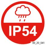
Protection rating IP54 (All over protection against dust and water spray).
