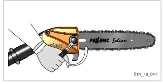
Re-position the handle of the telescopic wrench (11) on its holding magnet.
