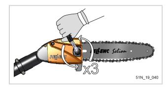
Tighten the chain guard lock nut (12) correctly using the telescopic wrench (11), the chain guide (13) then moves forward and automatically tensions the chain (14).
