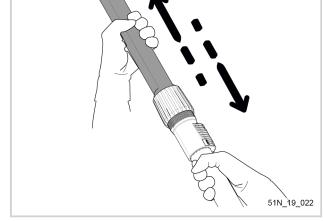
Tighten the pole locking nut (15).
