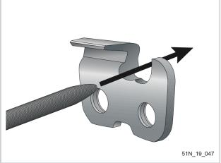
1. Hold the mark on the file holder parallel with the mark on the platen. Proceed in the opposite manner for the other side.
