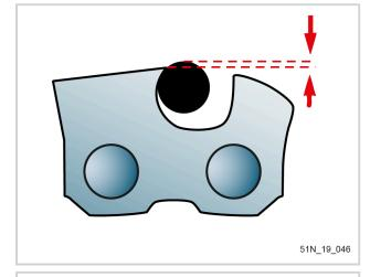
Sharpen the cutters from one side of the chain by filing from the interior toward the exterior. Only file by pushing.
