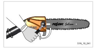
3. Re-position the handle of the telescopic wrench (11) on its holding magnet.
