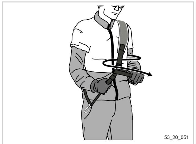
5. Mount the carrying eyelet on the tool pole.
