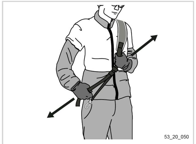
3. Pass the end of the strap which is self-attaching under the main strap.
