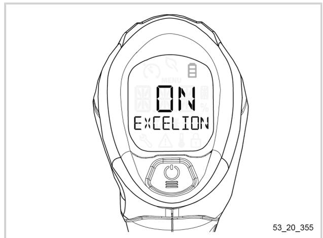
3. Make sure the screen displays the name of the battery.
