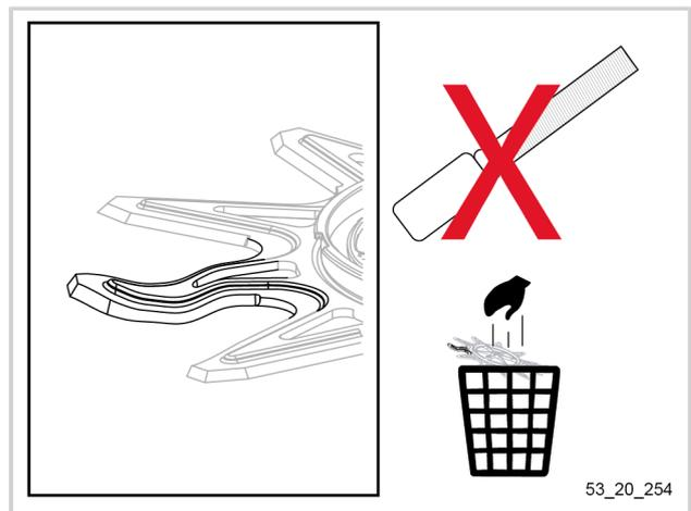
2. Proceed with the sharpening of the blade, taking care to maintain an inclination of 45° between the blade and the file.
