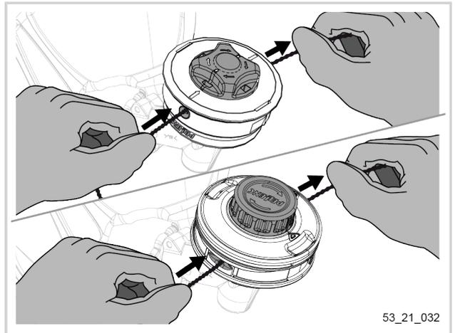
The strimmer wire should be the same length on both sides of the cutting head.
