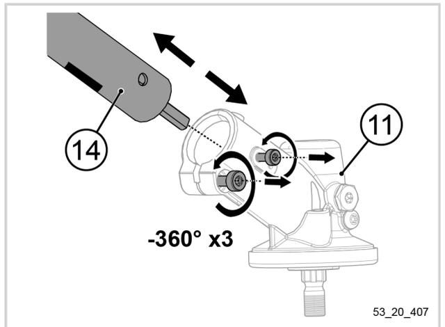
4. Unscrew the two screws on the CITY CUT using the TORX 25 (22) wrench supplied with your tool.
