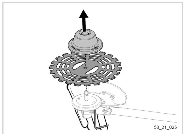
**Removing the cutting head**
