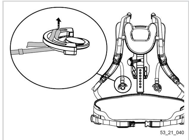
2. Fit the male chest buckle of the carrying strap in place of the original male chest buckle of the harness.
