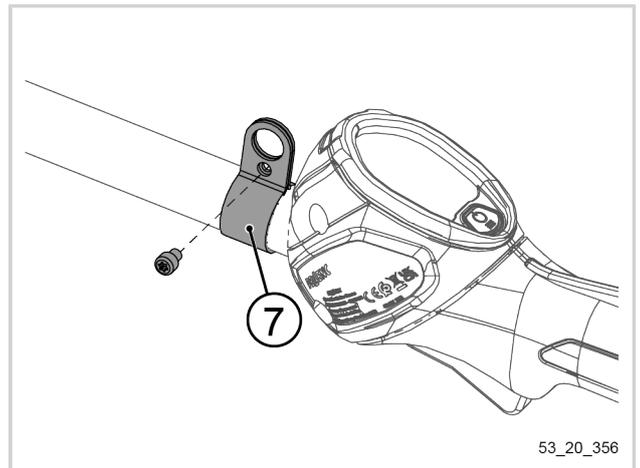
2. Slide the carrier ring over the transmission shaft.
