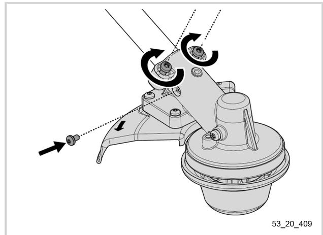
7. Align the angle gear and its cover in order to match the holes located on each of the elements.
