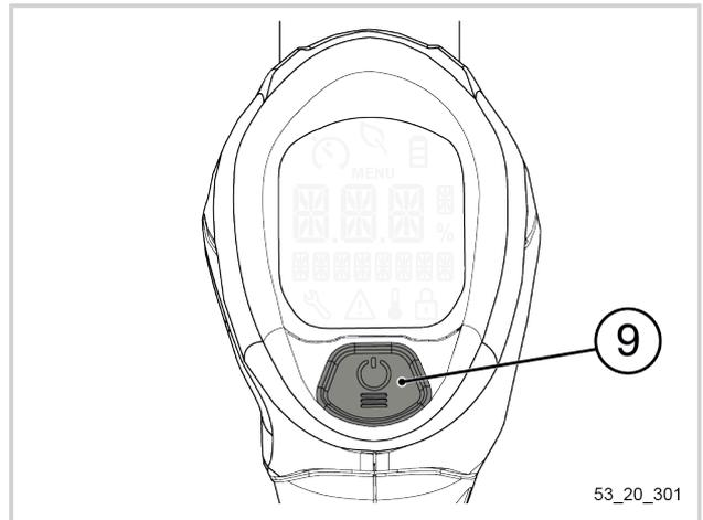
2. Make sure the tool turns on. The screen lights up in blue.
