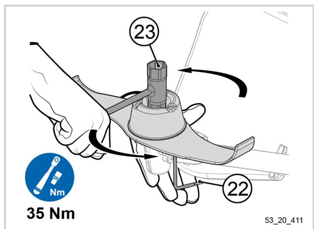
Fitted with the protective shield and the mulching blade, the brush cutter is ready for use.
