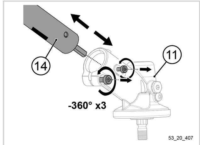
4. Remove the screw located on the right side of the angle gear supplied with your saw Kit (ref. 57275).
