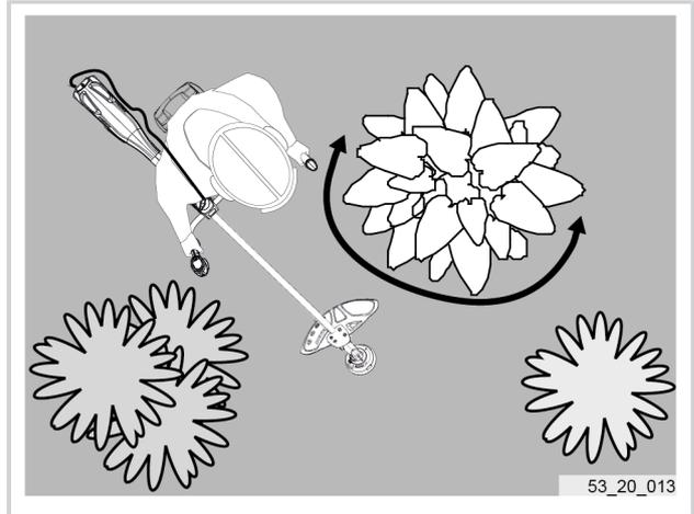
**Working with the clearing saw**
