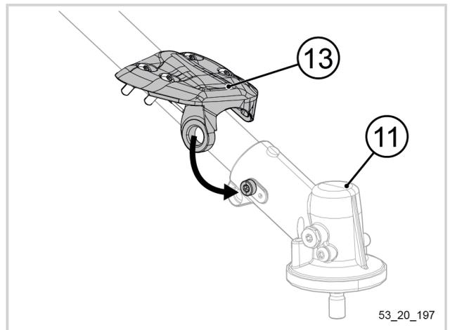
2. Fit the lower part of the safety guard (13) by aligning the screw marks.
