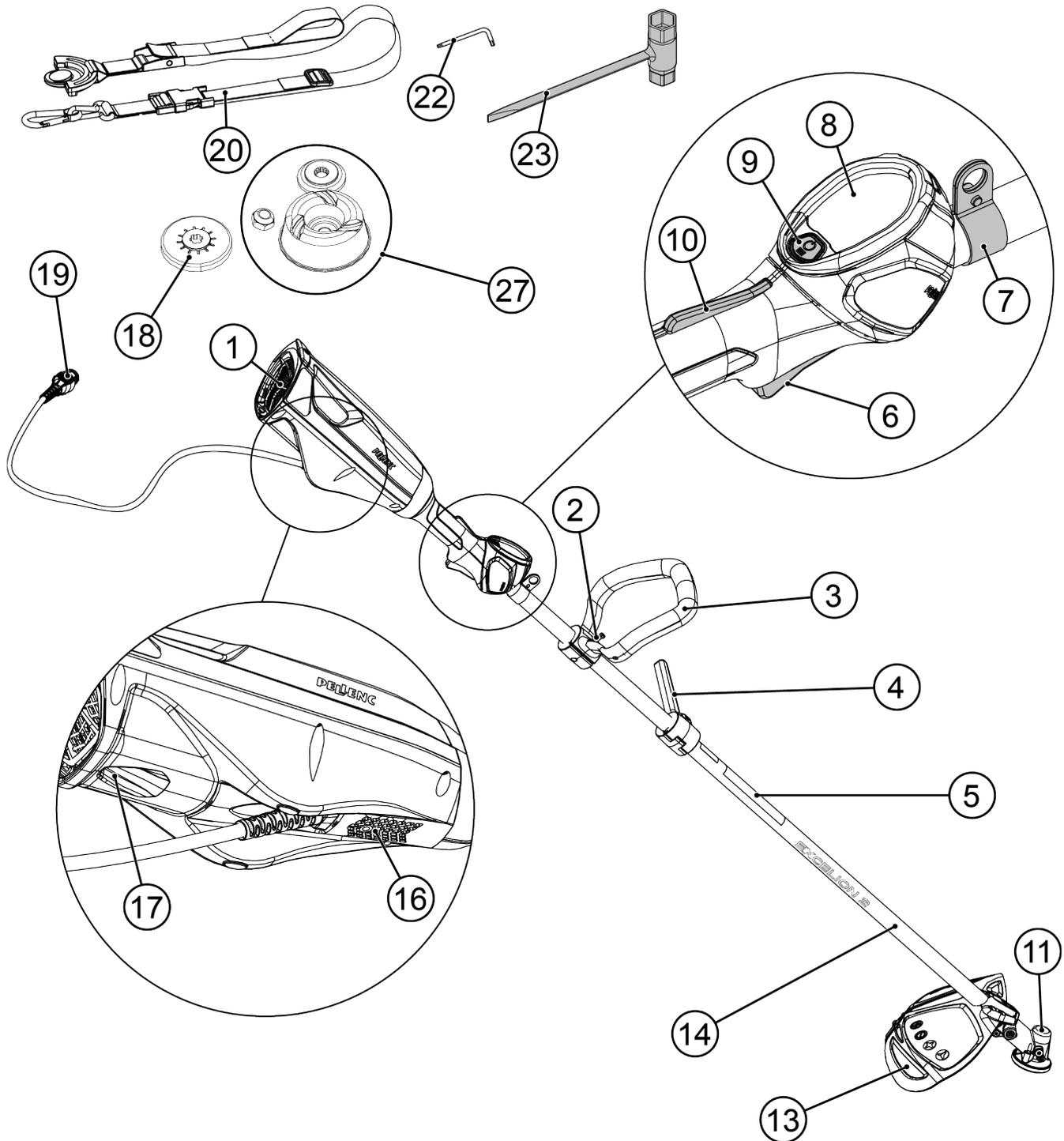
1. Air exhaust screen: A hot air discharge screen that cools the motor and the electronic board.
