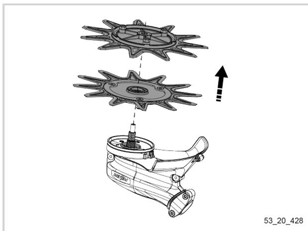
4. On each of the blade supports, using a TORX 27 screwdriver, remove the 3 nuts to separate the blade from its support.
