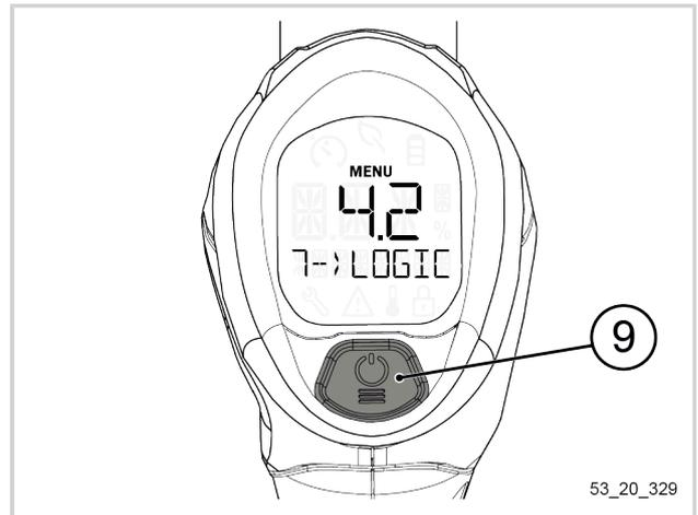
**- 5.5.3.8. DISPLAYING THE SOFTWARE VERSION OF THE MOTOR BOARD**
