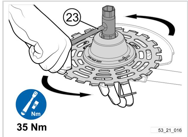
**Removing the chisel-saw blade**
