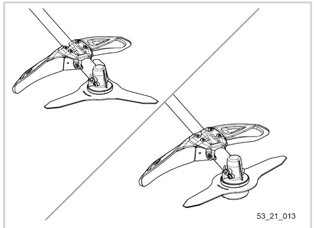
**Dismounting the tri-blade/twin-blade from the tool**
