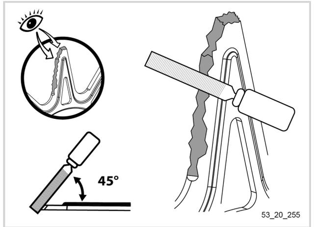
Always keep a distance of 3.7mm between the edge and the relief on the blade.
