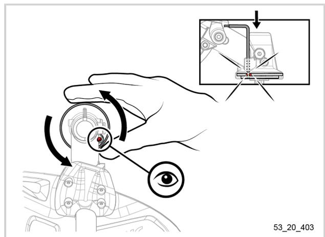
6. Tighten the head counterclockwise to lock the position.
