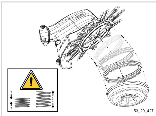
3. Remove the two blades each positioned on a support.
