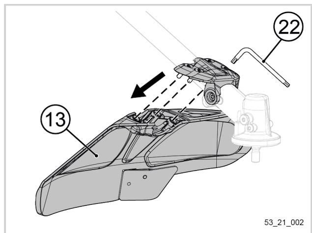
3. Remove the upper part of the safety guard (13) by first removing the eyelet fitted on the upper screw of the angle gear (11).
