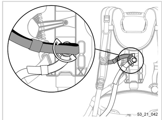
3. Fit the carrying strap end buckle in the location provided on the harness, making sure to pass over the harness holder.
