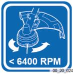
Be sure to check the direction and speed of rotation of the cutting head.
