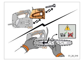
Before the first use, check the voltage of the chain (See the procedure of Checking the tension of the chain). If the chain is slack, refer to the chain tension explanations (see procedure Section 6.5, "Automatic chain tension").
