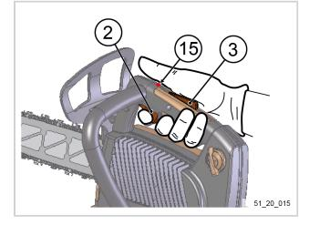
5. Release the trigger (2) to stop the motor.
