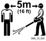
Nobody must stand within 5 m (16ft) of the tool in operation.
