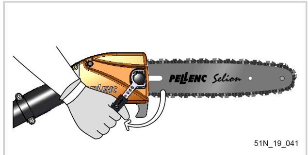
3. Re-position the handle of the telescopic wrench (11) on its holding magnet.
