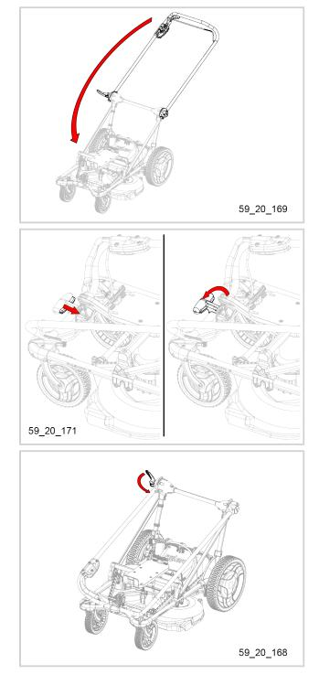
7. Lock the cutting height adjustment handle (16).
