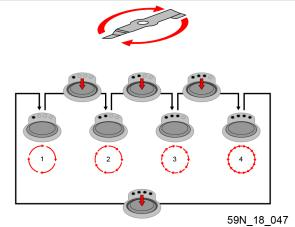
Even if the cutting blade speed is cut because the optical sensor is dirty, you can still carry on working by manually setting one of the 3 blade rotation speeds. The density sensor will no longer regulate the blade rotation speed automatically.
