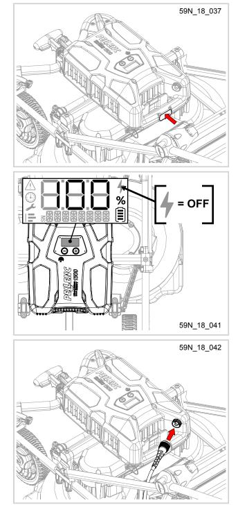
Before electrically connecting the battery to the mower, check that the battery power indicator is off.
