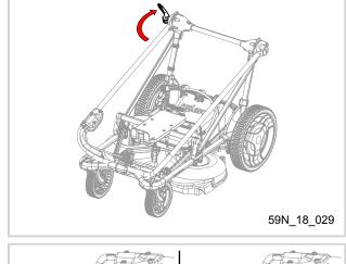
With one hand, hold the cutting height adjustment handle (16) while simultaneously pressing on the two buttons to release it from its position.
