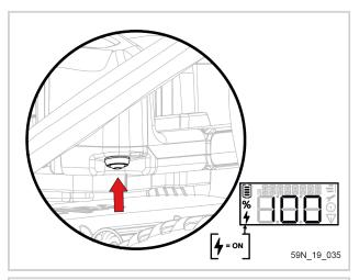
260 / 520 Alpha battery: Switch on the battery by pressing the Alpha 260/520 battery support tray push button.
