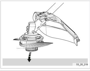
The strimmer wire length will be gradually adjusted by cutting itself on the blade of the safety guard.
