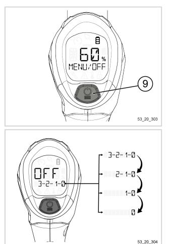
The screen displays "OFF" and there is a countdown, until the tool comes to a complete stop.
