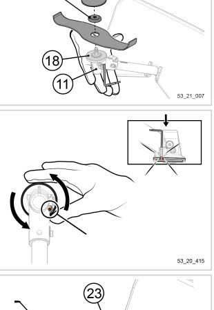
6. Using the special EXCELION 2 wrench (23) supplied with your tool, tighten the nut anti-clockwise while holding the protective bowl.
