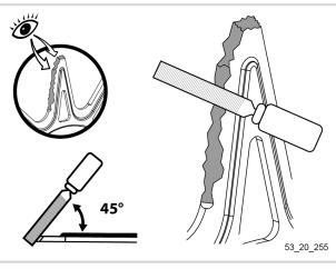
Always keep a distance of 3.7mm between the edge and the relief on the blade.
