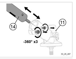
4. Unscrew the two screws on the CITY CUT using the TORX 25 (22) wrench supplied with your tool.
