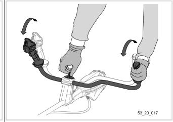
3. When the user has found a suitable position, screw in the handle adjustment knob (2) while exerting downward pressure, firmly holding the left handle grip of the tool.
