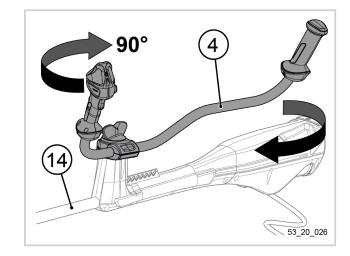
2. To adjust the handle, adjust the arm-handle distance by bringing it back towards the user or, alternatively, by pushing it towards the front of the machine.
