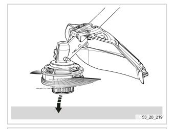
The strimmer wire length will be gradually adjusted by cutting itself on the blade of the safety guard.
