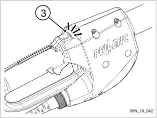
5. Lift the Soil Cultivator so that it is not touching the ground when starting up.
