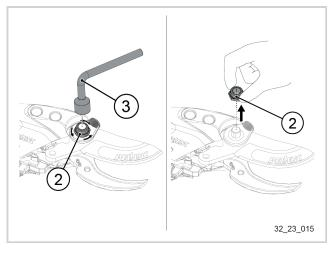
5. Loosen the nut (2) with the key provided (3).
