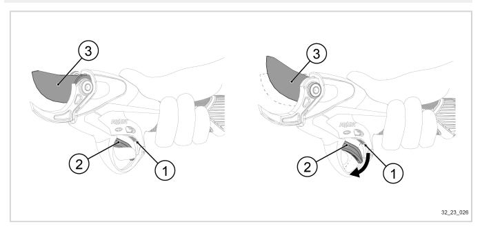
The blade (3) remains in half-open position as long as the optical sensor (1) detects that the user's finger is in front of the trigger (2).
