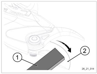
8. Check the tightness of the blade. See 6.3.6. Adjusting the tightness of the blade, page 38.
