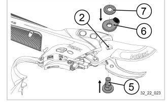
10. Position and screw the nut (8) onto the blade shaft (5) using the wrench provided (9), see Section 6.4, "Check the tightening of the blade".
