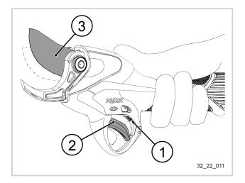
In half-open mode, the blade remains in half-open position as long as the optical system (4) detects that your finger is in front of the trigger (2). When your finger moves away from the trigger, the optical system controls the full opening of the blade (3).
