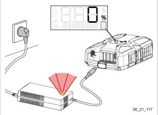
6. Connect the charging cord (18) to the battery's charging connector (4). The battery beeps twice when it recognizes the charger, the charger light turns green blinking green after a few seconds
