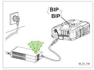
7. The battery is charging: The charger LED lights up green and flashes. The segments of the charging indicator flash in sequence.
