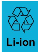
Marking symbol for identifying the chemical characteristic of the battery during recycling.
