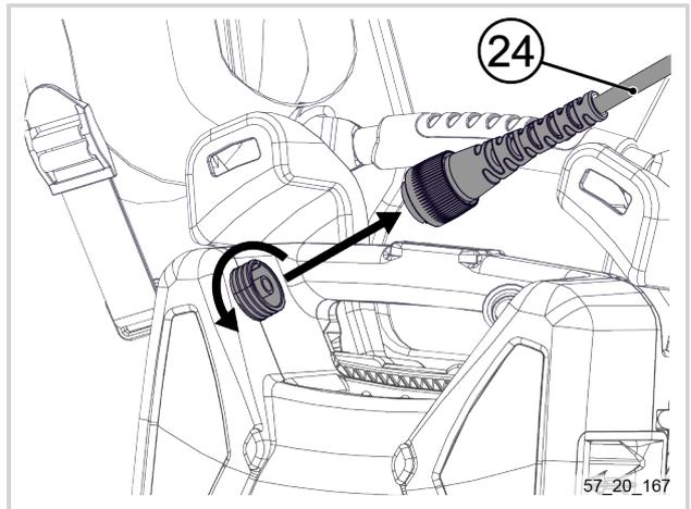
5. Remove the battery from the harness (see harness assembly instructions).
