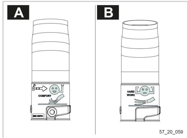
2. Fit the ergonomic elbowed nozzle (17) onto the end
