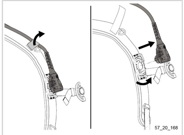
3. Unscrew the connector safety ring to release the extension cord.
