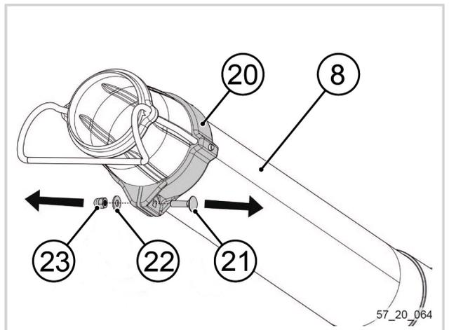
2. Remove the assembly from the outlet blowing nozzle (8).
