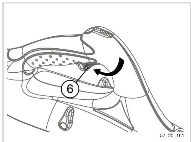
6. Release the trigger (6) to stop the tool
