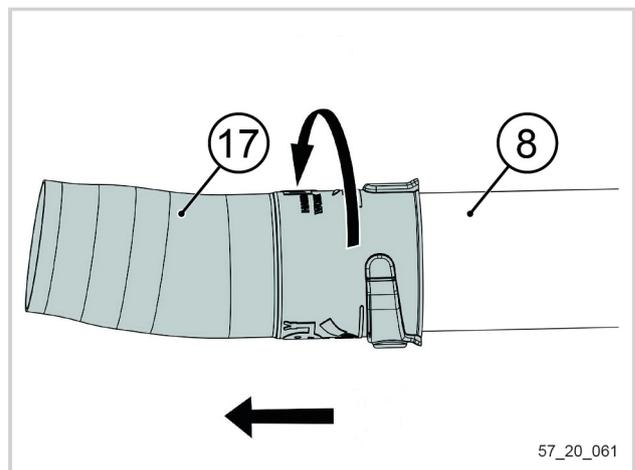
**4.4. FITTING/REMOVING THE BLOWER SCRAPER (OPTIONAL)**
