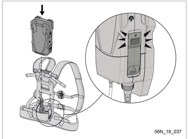
2. Connect the extension cord connector to the harness.
