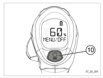
The screen displays "OFF" and there is a countdown, until the tool comes to a complete stop
