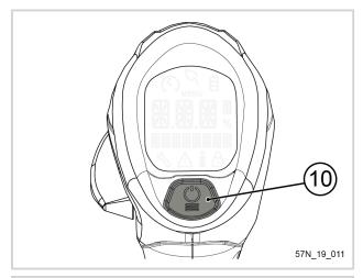
3. Make sure the tool turns on. The screen lights up in blue.
