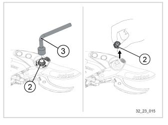
5. Loosen the nut (2) with the key provided (3).
