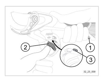
Check the correct operation of the blade according to the position of the trigger (2).
