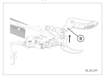
8. Remove the blade (9) and dispose of it.
