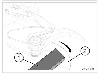
8. Check the tightness of the blade. See 6.3.7. Check the tightness of the blade, page 40.
